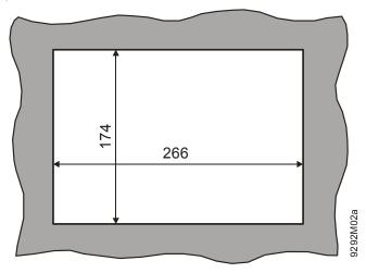
Wall thickness: 1 mm to 4 mm
