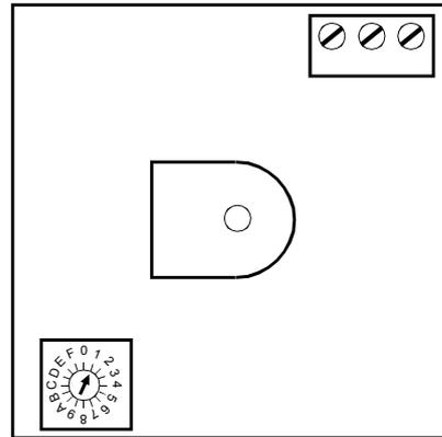
Address switch inside the housing.
