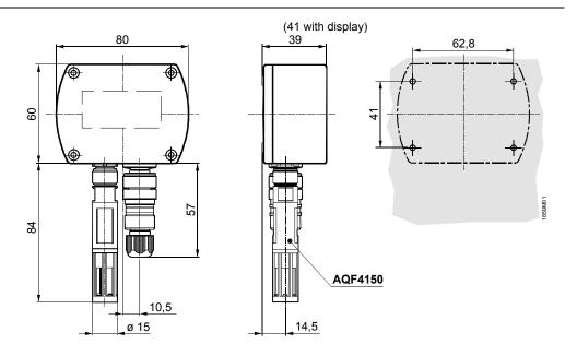
Dimensioning without (with) LCD-display
