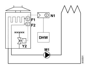
wall-hung boiler with independent control of DHW
