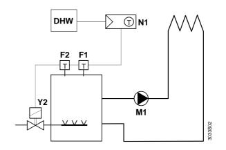
Room temperature controller with direct control of a gas-fired Room temperature controller with direct control of a gas-fired floor-standing boiler with independent control of DHW
