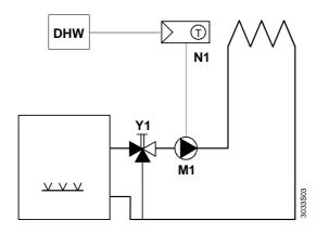
Room temperature controller with direct control of a heating circuit pump (precontrol by manual mixing valve) with independent control of DHW
